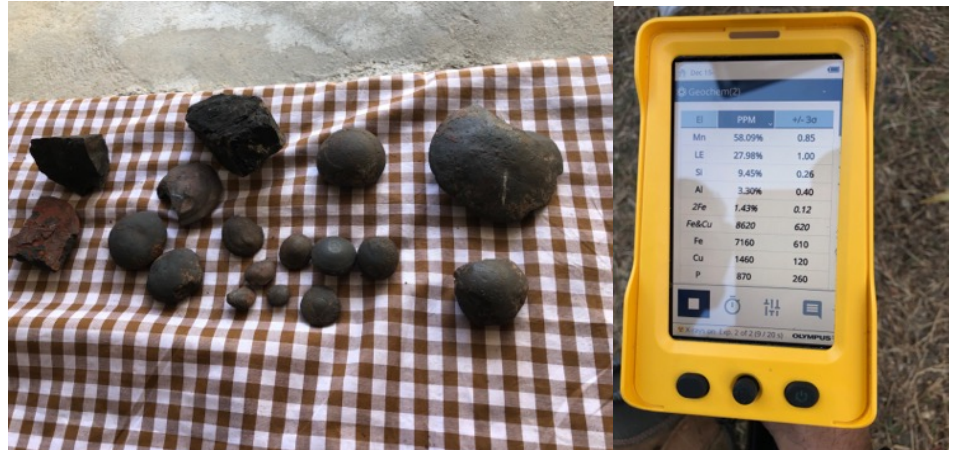
Figure 5.2 – Manganese Nodules Samples and XRF Reading (Mn 58%)
