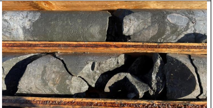
Massive & breccia chalcocite (dark grey) from 36m downhole in drill hole ST22-01
