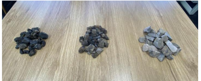
Left to right: Very High Density product 53.9% Cu (DSO), High Density product 10.3% Cu, and Low Density product 0.3% Cu (waste rock) portable XRF results
