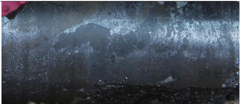
Figure 5.4 – High grade massive galena and sphalerite (SHDD0001, 228.6m)
